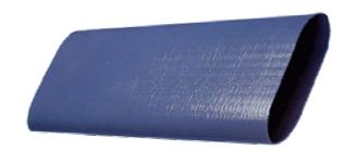
The Model PD1 is a blue PVC discharge lay-flat hose that resists kinking and twisting. It is designed as a standard duty hose for water discharge in industrial and construction applications, is strong and economical, and rolls up flat for easy storage. Reinforcement includes spiral plies and longitudinal synthetic cords for excellent burst resistance. Other varieties for higher pressures alternate materials are also available.
